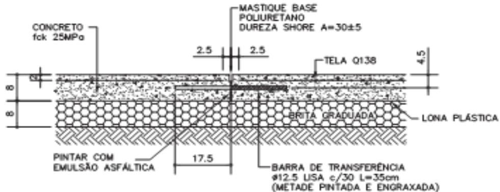
JUNTA DE CONSTRUÇÃO (C)
