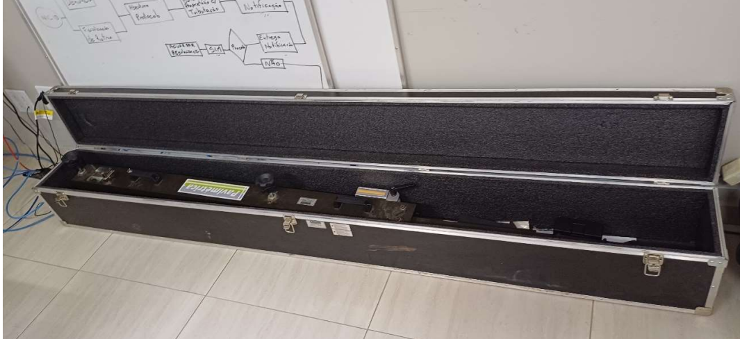
VIGA BENKELMAN_2:1 COM EXTENSOMETRO DIGITAL
